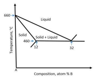
The freezing range of the alloy with 16% B is \_\_\_\_\_ (in °C to one decimal place)
