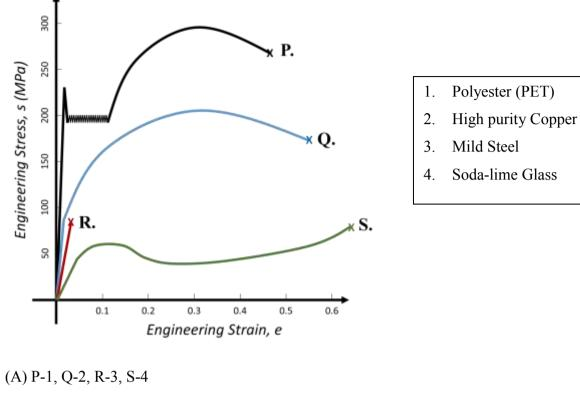
Q.31 Match the four tensile stress-strain curves (P,Q, R, S) with the materials listed in the box:
