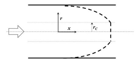
Consider r and x as the radial and axial directions, and the shear stress is finite as r approaches zero. A force balance results in the following equation
