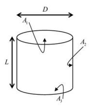
$F_{ij}$  denotes the fraction of radiation energy leaving the surface  $A_i$  which reaches the surface  $A_j$ . It is also known that  $F_{13}=3-2\sqrt{2}$ . Which one of the following is correct?
