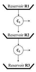
The efficiencies of the engines  $C_1$  and  $C_2$  are 0.40 and 0.35, respectively. If the temperature of Reservoir R1 is 800 K, then the temperature (in K) of Reservoir R3 is \_\_\_\_\_ (round off to nearest integer).
