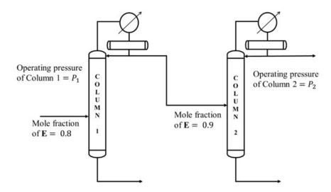
Mole fraction of E in the distillate obtained from column 1 is 0.9. If the column pressures  $P_1$  and  $P_2$  are in kPa, which one of the following is correct?
