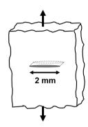
Q.14 A unidirectionally aligned carbon fibre reinforced epoxy composite is loaded as shown in the figure. The volume fraction of the fibre is 0.6. The Young's modulus of the composite is \_\_\_\_\_ GPa.
