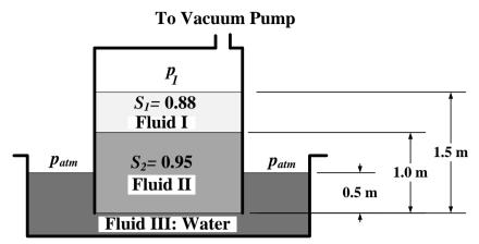
Unit weight of water,  $\gamma_w = 9.81 \text{ kN/m}^3$ Atmospheric Pressure,  $p_{atm} = 95.43 \text{ kPa}$
