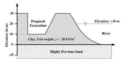
The water level in the adjacent river is at an elevation of +20.0 m. Unit weight of water is  $10 \text{ kN/m}^3$ . The factor of safety (up to two decimal places) against sand boiling for the proposed excavation is \_\_\_\_\_
