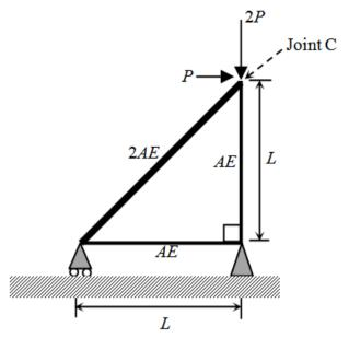
Given that  $E = 2 \times 10^{11} \text{ N/m}^2$ ,  $A = 10 \text{ mm}^2$ , L = 1 m and P = 1 kN. The horizontal displacement of Joint C (in mm, up to one decimal place) is \_\_\_\_\_
