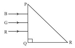
The refractive indices of the material of the prism for red, green and blue wavelength are 1.27, 1.42 and 1.49 respectively. The colour of the ray(s) emerging out of the face PR is:
