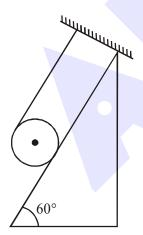
[The coefficient of static friction,  $\mu_s$ , is 0.4]
