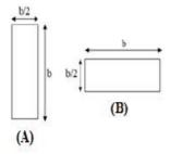
Bending moments applied to the beam in both cases are the same. The maximum bending stresses  $(\sigma)$  induced in cases (A) and (B) are related as
