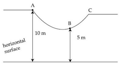
As shown in the figure, a particle of mass 10 kg is placed at a point A. When the particle is slightly displaced to its right, it starts moving and reaches the point B. The speed of the particle at B is x m/s.
