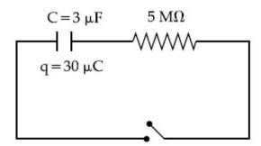
The circuit shown in the figure consists of a charged capacitor of capacity 3  $\mu F$  and a charge of 30  $\mu C$ . At time t=0, when the key is closed, the value of current flowing through the 5  $M\Omega$  resistor is 'x'  $\mu A$ .
