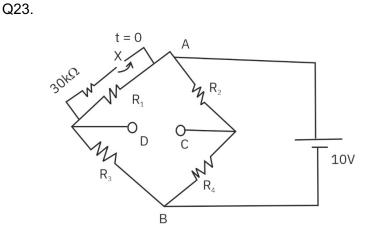
In a given Wheatstone bridge. R1 = 1.5 k  $\Omega$ , R2 = R3 = R4 = 1k  $\Omega$
