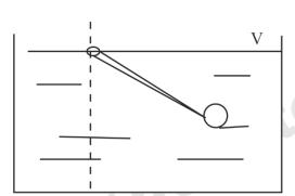
A uniform wooden rod (sp gravity = 0.6, dia – 4 cm and  $\ell$  = 8 m) is immersed in the water and is hanged w\o friction at point A on the waterline as shown in the fig. A solid spherical bal made of lead (sg<sub>L</sub> = 11.4) is attached to the free end of the rod to keep the assembly in static equilibrium inside the water. For simplicity assume that the radius of the ball is much smaller than the length of the rod.
