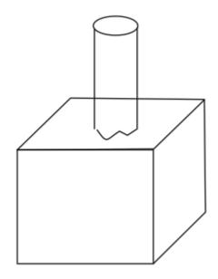
Cylindrical riser is placed at top of casting and is insulated to top
