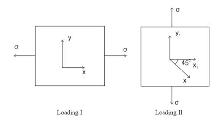
TATY .com A linear elastic structure under plane stress condition is subjected to two sets of loading I & II. The resulting states of stress at a point corresponding to there two loading are as shown. If there two sets of loading are applied simultaneously then the net normal component of stress  $\sigma_{xx}$  is:
