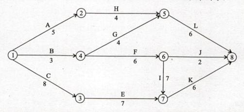
Convert the given A-O-A (Activity on Arrow) to A-O-N (Activity on Node) Network and indicate the critical path. The duration of each activity is shown in the figure. 10
