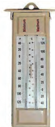
Fig 2.2 : Minimum and maximum thermometer
