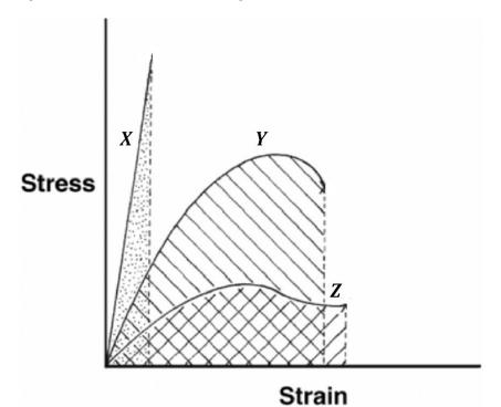
X – Titanium, Y – Hydroxyapatite, Z – Polyethylene
