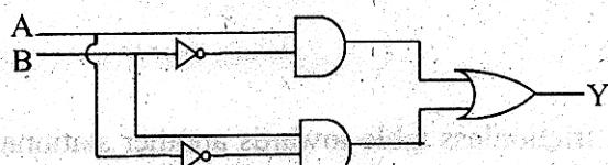
For the given logic circuit, the output Y for inputs  $(A = 0, B = 1)$  and  $(A = 0, B = 0)$  respectively are
