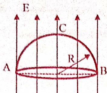
A hemisphere of radius  $R$  is placed in a uniform electric field  $E$  so that its axis is parallel to the field. Which of the following statement(s) is / are true ?
