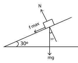
Balancing force invertical  $N \cos 30^\circ - mg - \mu N \cos 60^\circ = 0$   $N(\cos 30^\circ - \mu \cos 60^\circ) = mg$  $\Rightarrow N = \frac{mg}{(0.87 - 0.2 \times 0.5)} = \frac{8000}{0.77} = 10.4 \times 10^3 \text{ N}$
