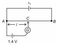
In the shown potentiometer the cell of emf 1.4 V is balanced at point C, 60 cm away from A. Then  $\varepsilon_0$  is equal to (AB = 3 m)
