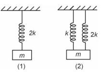
The ratio of time period of oscillation of system (1) to that of system (2) is
