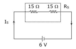
Effective resistance of the circuit,  $R_S = R_1 + R_2$
