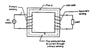
Construction: It consists of the separate coils of insulated wire wound on same iron care one of the coil connected to a.c. input is called primary (p) and the other winding giving output is called secondary (s) coil.
