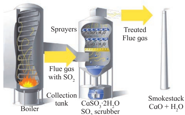
Fig. 15.5 : Exhaust gas Scrubber
