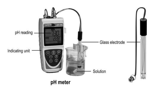
To measure the pH of a solution, the glass electrode is dipped into the solution and the pH is displayed on the screen of the indicating unit. Before measuring the pH of another solution, the glass electrode is rinsed with distilled water and dried carefully with tissue paper.
