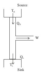
$$1 - \frac{Q_{L}}{Q_{H}} = 1 - \frac{T_{L}}{T_{H}}$$
