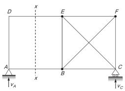
Shear force at x-x = Panel shear force =  $V_A$  There is no member to resist panel shear force. So unstable.
