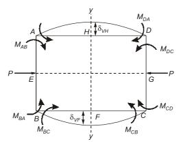
Shear forces at H and F are zero since it is subjected to pure bending. Horizontal displacements at H and F are zero since axial deformations are neglected. At the axis of symmetry, slopes must be zero for the deflection profile to be symmetrical. .: Slopes at *E*, *F*, *G*, *H* are zero.
