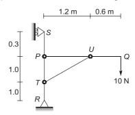
The horizontal component of force transferred from horizontal member PQ to the vertical member RS at P is \_\_\_\_\_.
