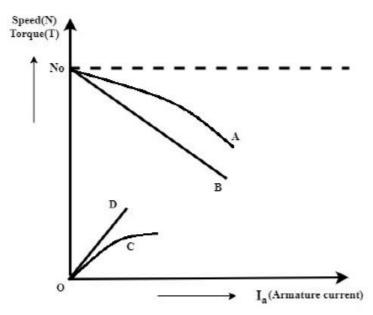
Which of the above curves represent N versus Ia and T versus Ia respectively with armature reaction neglected?
