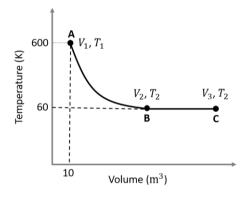
$A \to B$  is an adiabatic process. If the total heat absorbed in the entire process  $(A \to B \text{ and } B \to C)$  is  $RT_2 \ln 10$ , the value of  $2 \log V_3$  is \_\_\_\_.
