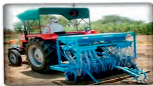
Fig. 5.6 : drilling by tractor drawn implement
