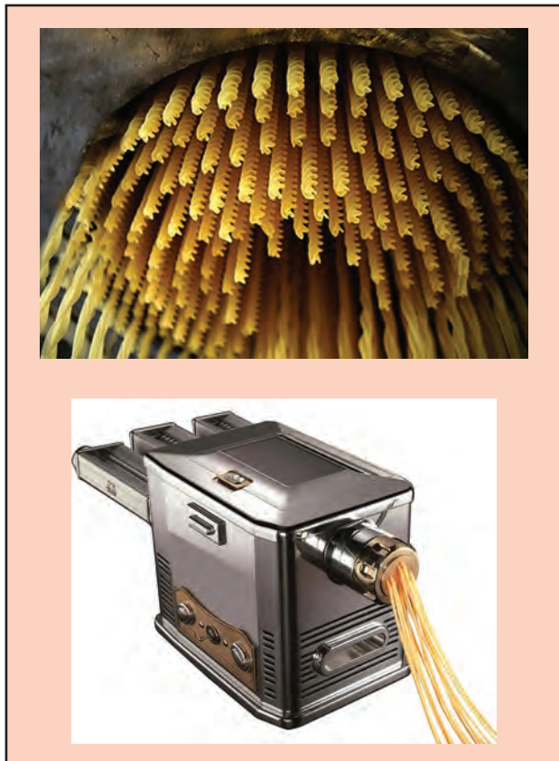
Fig. 10.3a : Pasta making machine (Extrusion of Pasta)
