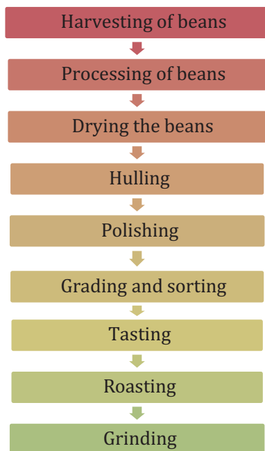
Fig. 12.20 Flow chart of coffee production
