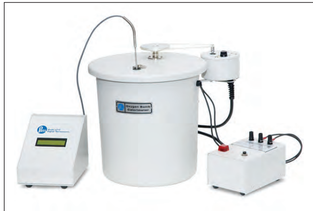
Figure 5.1 : Diagram of bomb calorimeter
