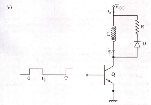
For the figure shown above, the transistor 'Q' is excited by a pulse of duration ' $t_1$ ' with a periodicity of  $\frac{1}{T}$ .
