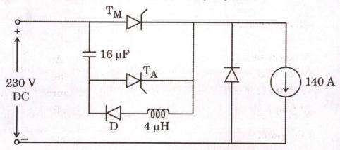
where  $T_{M}$  is main thyristor and  $T_{A}$  is Auxiliary thyristor.
