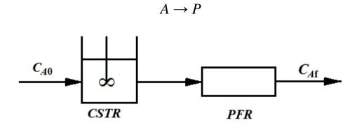
The rate constant is  $0.2 \text{ s}^{-1}$ . The space-time is 5 s for both the reactors. The overall fractional conversion of *A* is \_\_\_\_\_\_ (rounded off to third decimal place).
