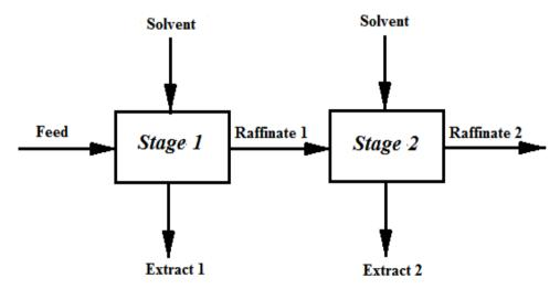
Components **B** and **C** are immiscible. 60% of **A** in the feed is extracted in **Stage 1**. The equilibrium relation is given by  $Y^* = 1.5 X$  where,
