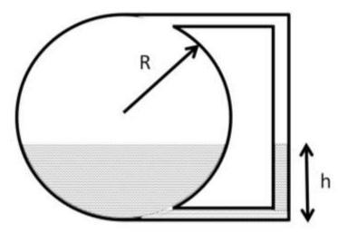
The estimate of liquid height (in m) to store  $V = 30 \text{ m}^3$  of water in R = 3 m tank, after performing ONE iteration of Secant method, using 1 m and 3 m as two initial guesses of liquid height is \_\_\_\_\_\_ (rounded off to second decimal place).
