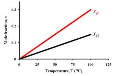
If the yield of Q based on reactant P consumed  $(Y_Q)$  at 25 °C was found to be 0.40, then the value of  $Y_Q$  at 60 °C is \_\_\_\_\_ (rounded off to second decimal place).
