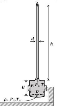
Q.16 Considering the air flow to be streamline, the steady mass flow rate of air exiting the chimney is \_\_\_\_\_ gm s<sup>-1</sup>.
