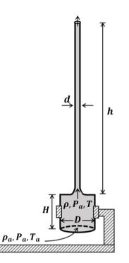
Q.17 When the chimney is closed using a cap at the top, a pressure difference  $\Delta P$  develops between the top and the bottom surfaces of the cap. If the changes in the temperature and density of the hot air, due to the stoppage of air flow, are negligible then the value of  $\Delta P$  is \_\_\_\_\_ N m<sup>-2</sup>.
