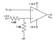
Which one of the following correctly represents the output  $V_{\mbox{\scriptsize out}}$  corresponding to the input  $V_{\mbox{\scriptsize in}}$  ?
