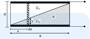
$$C_{eq} = \frac{C_1 C_2}{C_1 + C_2} = \frac{k \varepsilon_0 a dx}{k d + (1 - k) y}$$
