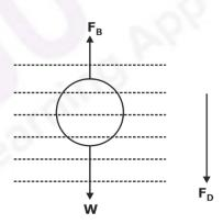
Drag force  $(F_D)$  = wt. of the sphere (W) - Buoyant force  $(F_B)$
