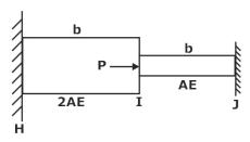
To make the axial force in rod HI equal to zero, the value of the external force P (in N) is \_\_\_\_\_\_. (round off to the nearest integer)
