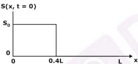
The boundary conditions of the problem are given by  $\frac{\partial s(x,t)}{\partial t}=0$  at the boundary point x=0 and x=L at all times. Consider D=0.1 m<sup>2</sup>/s.  $S_0=5$  µmol/m, and L=10,
