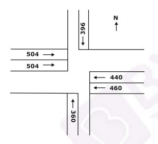
The optimum cycle length (in seconds), as per the Webster's method, is \_\_\_\_\_. (round off to the nearest integer)
