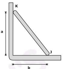
The minimum coefficient of static friction that is required at the point J to hold the rod in equilibrium is \_\_\_\_\_\_\_. (round off to three decimal places)
