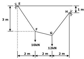
The magnitude of tension in the cable segment FG (kN, round off to two decimal places) is \_\_\_\_\_.
