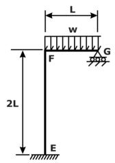
Considering the join F being rigid, the support reaction at G is
