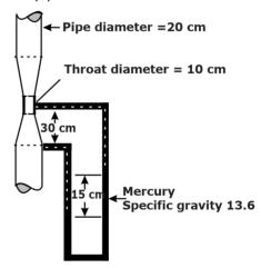
Assume  $g = 9.8 \text{ m/s}^2$ . When the deflection in the mercury manometer is 15 cm. the flow rate (in lps. Round of to two decimal places) considering no loss in the venturimeter is
