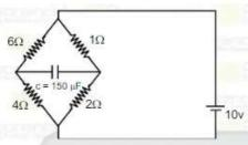
find charge on capacitor of 150 μF in steady state.
