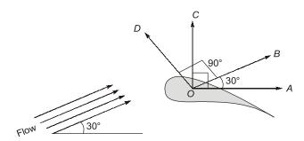
The direction of drag force on aerofoil is always along the direction of flow i.e. OB direction.
