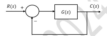
Consider the stable closed-loop system shown in the figure. The asymptotic Bode magnitude plot of G(s) has a constant slope of -20 dB/decade at least till 100 rad/sec with the gain crossover frequency being 10 rad/sec. The asymptotic Bode phase plot remains constant at  $-90^{\circ}$  at least till  $\omega = 10$  rad/sec. The steady-state error of the closed-loop system for a unit ramp input is \_\_\_\_\_ (rounded off to 2 decimal places).
