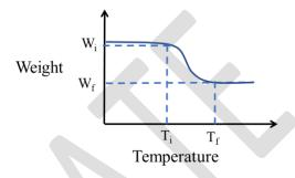
$W_i$  and  $W_f$  represent the weight of the material, corresponding to temperatures  $T_i$  and  $T_f$ , respectively. Which of the following factor(s) can influence  $T_i$  and  $T_f$ ?
