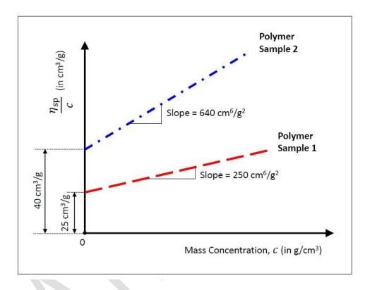
The ratio of the viscosity-average molecular weight  $(\overline{M}_v)$  of polymer sample 1 to that of polymer sample 2, i.e.,  $(\overline{M}_v)_1/(\overline{M}_v)_2$ , is \_\_\_\_\_\_ (rounded off to two decimal places).
