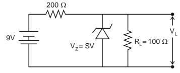
In the given circuit, find the voltage drop  $V_L$  in the load resistance  $R_L$ .
