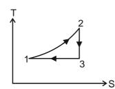
A cyclic process is shown in p-v diagram and T-S diagram. Which of the following statement(s) is/are true?
