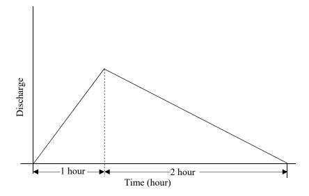
The peak discharge (in m<sup>3</sup>/s, rounded off to one decimal place) of the above unit hydrograph is \_\_\_\_\_
