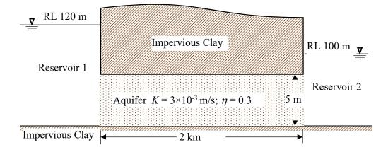
If the Reservoir 1 is contaminated by a pollutant then the time (in days, rounded off to one decimal place) taken by the pollutant to reach to the Reservoir 2 under advection will be
