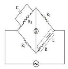
$$R = \frac{R_1 R_2}{R_3}, \qquad L = \frac{R_1 R_2}{C}$$
