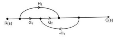
$\frac{c(s)}{R(s)}$  for the system shown in figure is
