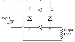
This figure represents the circuit of full wave bridge rectifier.
