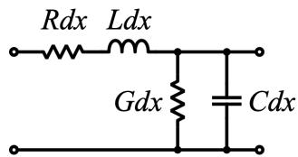
Suppose a two-wire transmission line has a basic element as represented above. Assume the special case of a lossless line where R=0 and G=0.
