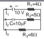
In steady state there will be no current in branch of capacitor, so no voltage drop across  $R_2 = 5\Omega$
