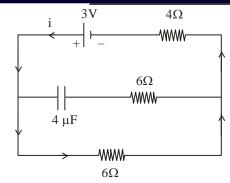
No current will flow in capacitor in steady state, current flowing in the circuit in steady state
