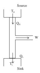
$$1 - \frac{Q_{L}}{Q_{H}} = 1 - \frac{T_{L}}{T_{H}}$$
