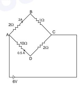
In steady state the capacitors will act as the open wire. Hence the circuit will be as above. If  $V_c = 0V$ then the potential at points A, B, C and D will be
