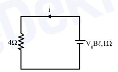
$$i = \frac{V_0 B \ell}{4+1} \implies V_0 = \frac{5(2mA)}{5 \times .2} = 10^{-2} \text{ m/s} = 1 \text{ cm/s}$$
