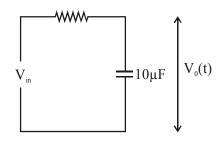
$$V_0(t) = V_{in} \left(1 - e^{-\frac{t}{RC}}\right)$$
