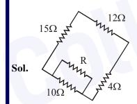
Let the resistance to be connected is R. For balanced wheatstone bridge,
